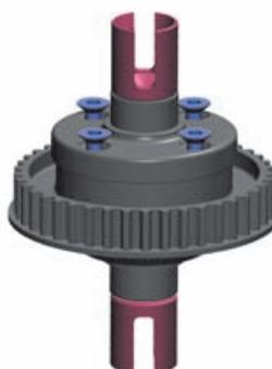
Tighten the screws equally but do NOT tighten them completely.
