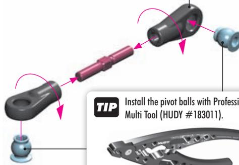
**TIP** Install the pivot balls with Professional Multi Tool (HUDY #183011).
