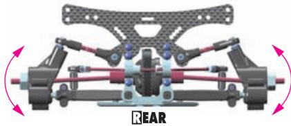
When the bars are set, verify that both sides move at the same time. If they do, the bars are set up correctly. If not, make sure that both downstops are the same and that the bar wire is flat.
