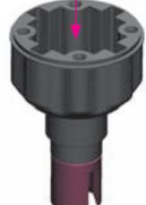
**TIP** Fill differential up to the top of the diff pins. DO NOT fill the diff to the top of the housing.
