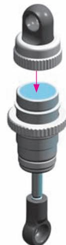
When installing the shock cap assembly on the shock body, some oil will leak out... this is normal.
