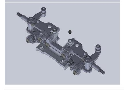
Time to install the front shocks. Start by installing the lower 3.55mm aluminum pivot balls on the shock piston side and screwing them onto the arm with an M2x6 BH Screw. Do this on both sides. It is a good idea to apply some 30,000 CST Grease or Oil for damping during this step.
