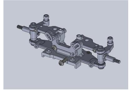
Now we will install the upper arms. Mount the arms by inserting the hinge pins with the flat spot towards the back and towards the top, through the arms and the bulkhead.
