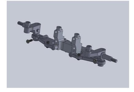
Start with the bottom arm installation on the bulkhead. Use the long dowel pins to mount the arms to the bulkhead by pressing them in. They are designed so that they will not fall out as they are tight on the arm and free on the bulkhead.
